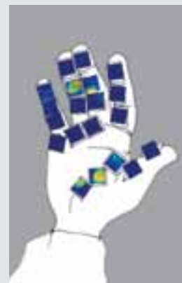
Force distribution Snowden-Pencer ring handle (large hand)
